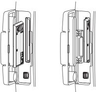
Figure 5.0a - Inserting C-CARD (details)
